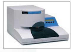
The Wallac DBS Puncher automatically punches dry blood spots into microtitration plates. It has a changeable head to allow the use of blood spots with diameters of 3.2, 4.7 or 6 mm. Two plates may be loaded to allow simultaneous preparation of different assays.
