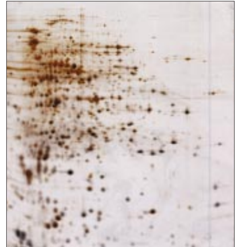
Fig 6. 2-D separation of an E. coli lysate. A 20-mg sample of E. coli lysate was separated on a 130 mm Immobiline DryStrip 3–10 L gel for the first dimension and a Hoefer SE 600 for the second dimension. First dimension separation was run for a total of 2 h 18 min (30 min at 500 V, 30 min at 1 000 V and 78 min at 8 000 V).
