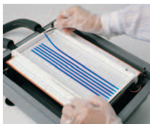
Align strips on the bed using the Immobiline DryStrip Kit
