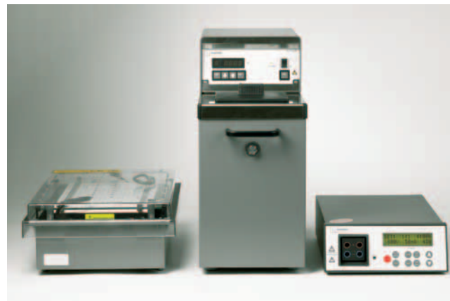
Fig 1. Main components of Multiphor II Electrophoresis System: Multiphor Electrophoresis Unit, MultiTemp III Throstatic Circulator and EPS 3501 XL Power Supply.
