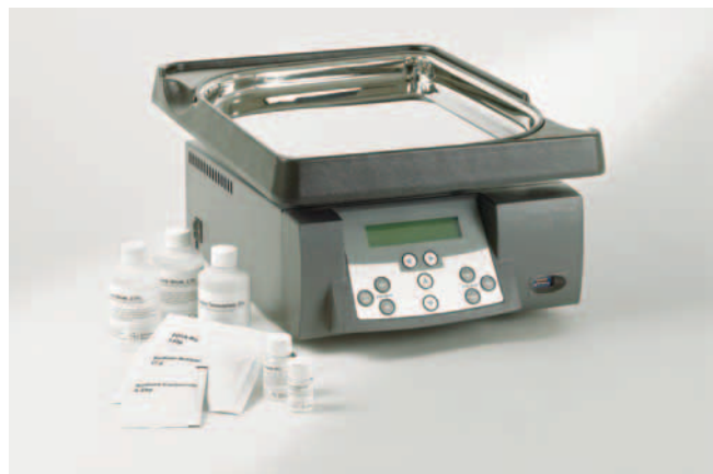
Fig 7. Processor Plus for automated staining and PlusOne Protein Silver Staining Kit
