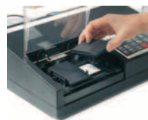
Fig 9. Simple blotting procedure of PhastTransfer.
