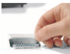
Fig 5. Applicator comb draws up identical sample volumes from droplets on a sample-well stamp.
