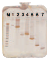
Analysis of crude PCR reaction products on PhastGel Homogeneous 12.5, silver stained.
